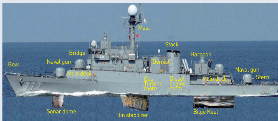
Figure 9. Overall shape and structures of ROKS Cheonan
